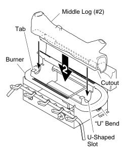
Figure 18 - Installing Middle Log (#2)
